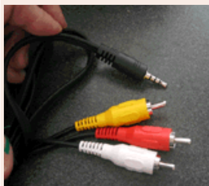
Figure 1. A camcorder A/V cable has a three-plug RCA connection at one end and a three-banded 1/8" plug at the other
