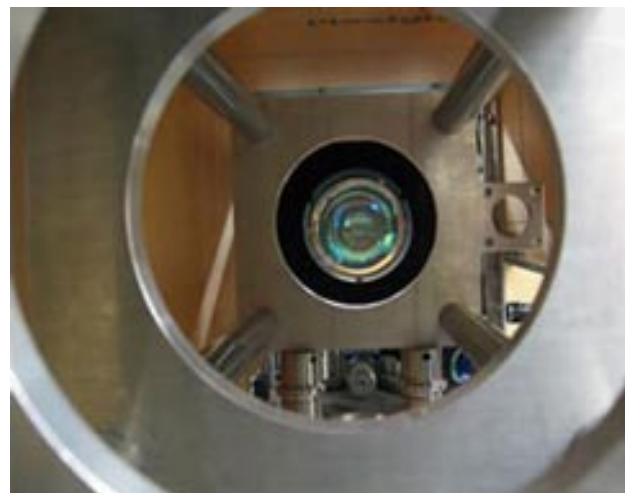
End-on view of high numerical aperture custom lens system used for trapping and imaging single atoms. (Image: Mark Saffman)
